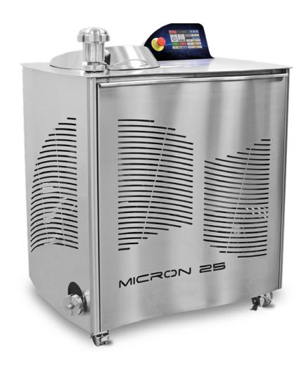
The Micron 25 ball refiner was designed for the production of spreadable creams, anhydrous pastes for ice creams, pralinated products and cream sweets. The machine is equipped with a refrigerator with the purpose of regulating, within the set limits, the excess heat caused by the friction generated between the spheres. Thus doing we preserve unaltered the organoleptic qualities of the product.
